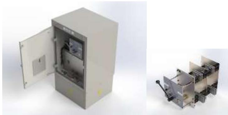
The Off Load Bypass Switch consists of a 2.0kA 1.5kV 2P Disconnecter in a bespoke enclosure. The Disconnecter has two positions, Open and Closed and each position has a volt-free microswitch, wired out to terminals, available for external use. The Disconnecter can be padlocked in both positions and the enclosure door can be padlocked closed.
