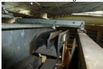
Conductor rail pick shoes on a depot trolley
