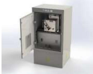
Howdon Depot switchgear for NEXUS, the Feeder Isolator Switch consists of a 2.0kA 1.5kV 2P Disconnecter in a bespoke enclosure. The Disconnecter has three positions, Earthed, Open and Closed and each position has a volt-free microswitch, wired out to terminals, available for external use. The Disconnecter can be padlocked in all three positions and the enclosure door can be padlocked closed.
